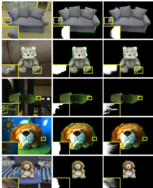
Fig. 9. The dataset used for quantitative comparison with [28], [8], [10]. First column: five of the input images (front views). Second column: our binary segmentation results in the first phase. Third column: our final results after matte refinement.
